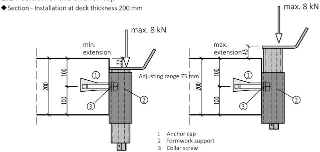
A stiff connection of the formwork elements must be ensured!
